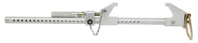
This fixed Beam anchor install on beams and other structural steel to create a stationary anchor point for a fall arrest device. They have two clamps that adjust to fit a range of beam sizes. A D-ring provides the attachment point. These devise can be removed and used in other locations. Anchors should always be inspected and replaced after being exposed to a fall.
