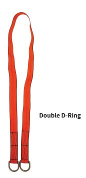
A Web Sling Anchorage is a type of anchorage device used in fall protection systems. It typically consists of a strong, flat webbing material with a loop or D-ring at one or both ends. The anchor is used to secure lifelines, lanyards, or other fall arrest equipment to a solid structure, providing a reliable point of attachment for workers at height.
